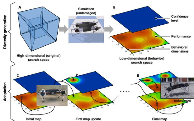
Fig. 1. **Concept of the IT&E algorithm** [6]. The first step occurs in simulation and aims at learning simultaneously thousands of high-performing gaits according to behavior dimensions. When an adaptation is needed on the real robot, a Bayesian optimization procedure searches in this map for the best gait. Picture adapted from [6].
