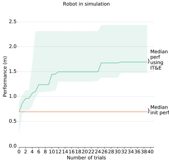
Fig. 2. **Best performance (covered distance) for each trial on the damaged robot in simulation.** The lines represent the median and the colored areas the 25<sup>th</sup> and 75<sup>th</sup> percentiles. The green color corresponds to the IT&E output performance. The orange line corresponds to the initial median performance, testing the best behaviors found in simulation. Each behavior is tested on a 10 seconds episode.
