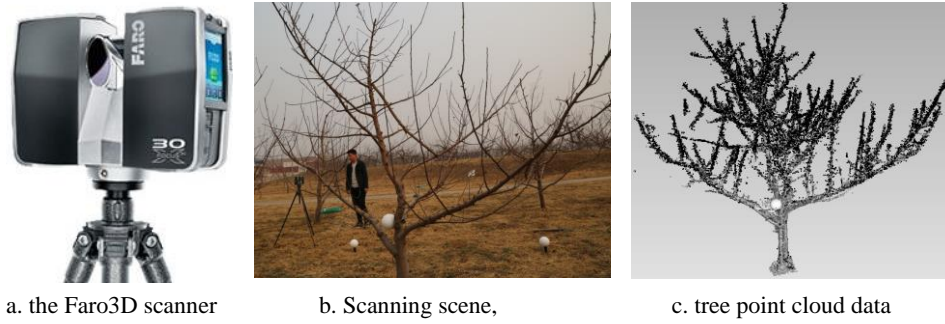
Fig. 4. The equipment and rule diagram of crown digitizer
