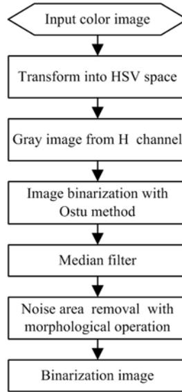
**Fig. 2.** The flowchart of trap image preprocessing
