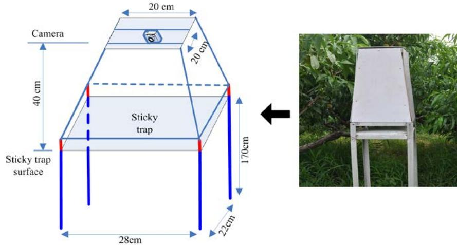
**Fig. 1.** Structure of insect trap
