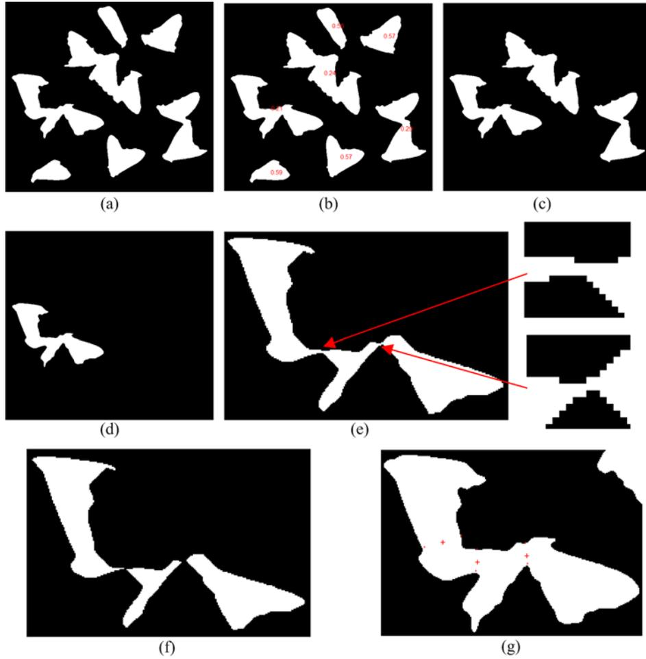
**Fig. 7.** Example of the local separation points search. (a) binary image after image preprocessing, (b) result of shape factor calculation, (c) all detected touching regions, (d) one of touching regions, (e) result after boundary stripping with 10 times, (f) result after boundary stripping with 11 times, and (g) results of local separation points search for one of touching region
