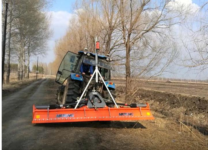
**Fig. 3b** The self—balancing adjustment of the graders
