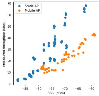
Fig. 6: Average E2E throughput with respect to RSSI.
