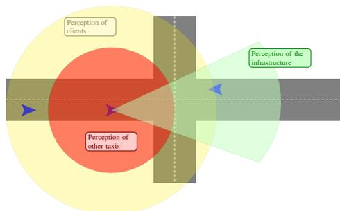
Figure 1: Different perception halos for a vehicle
