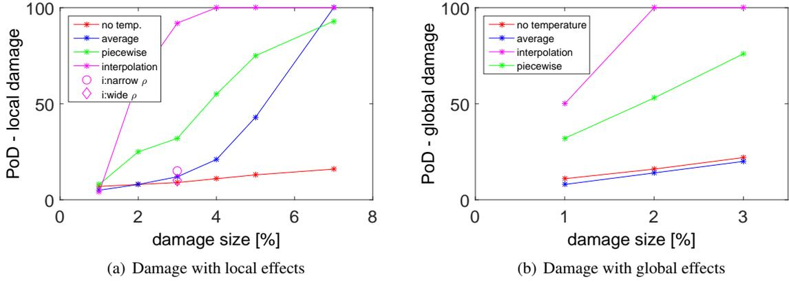
**Figure 5:** Probability of detection wrt. the damage size for different damage types.
