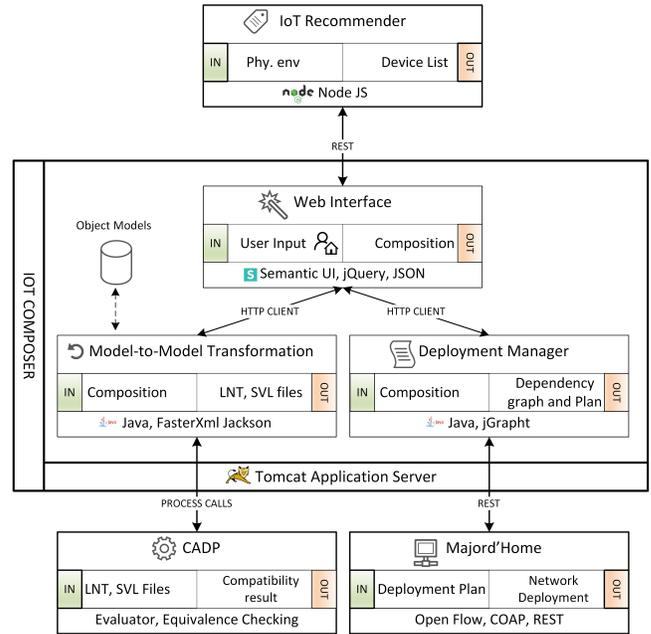
Fig. 3. Tool components and integration with various services.
