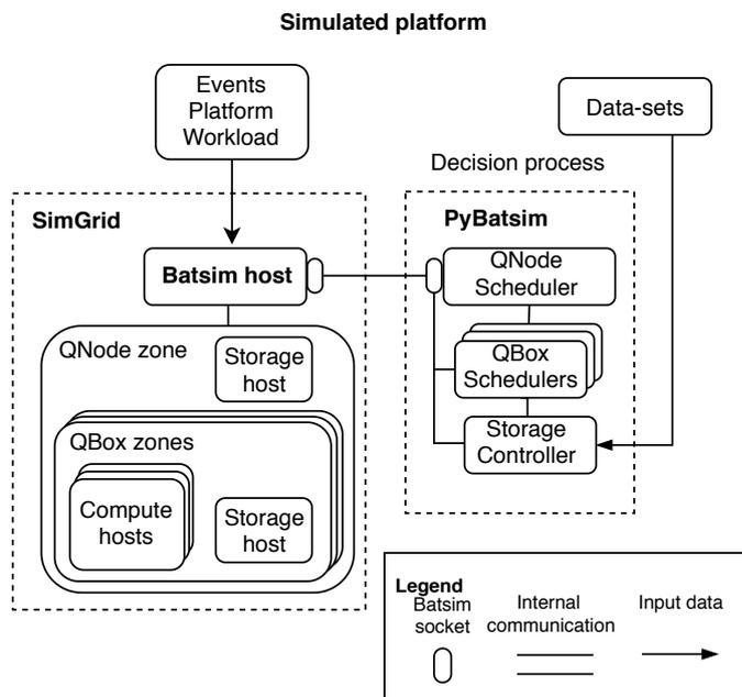
Figure 2: Scheme of the simulated Qarnot platform.
