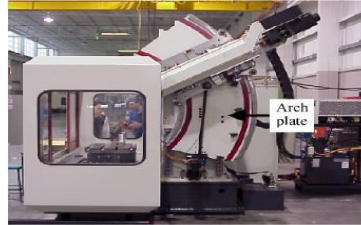
Fig. 1. Reconfigurable machine tool (RMT) developed at the ERC-RMS [4]
