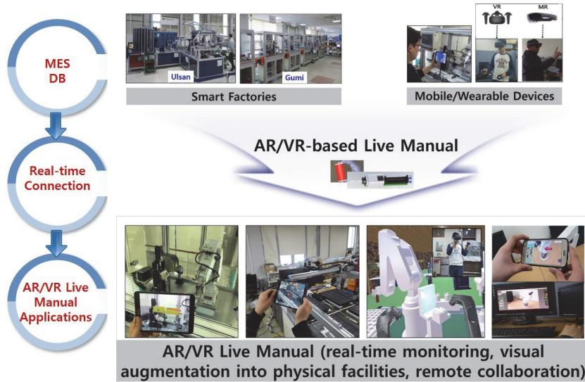
**Fig. 1.** Proposed AR/VR Live Manual for supporting various kinds of user-centric task assistance.
