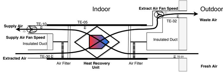
Fig. 1: Schematic diagram of air handling unit
