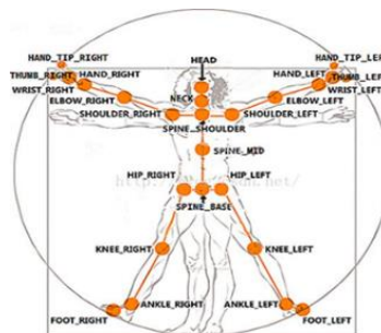
Fig. 1. Human skeleton structure defined by Kinect
