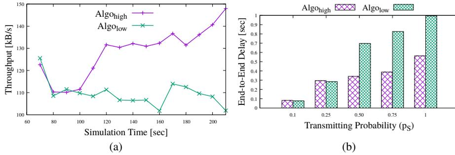
**Fig. 4.** The throughput (Figure 4(a)) and the end-to-end delay (Figure 4(b)) indexes comparing *Algo<sub>high</sub>* and *Algo<sub>low</sub>*.
