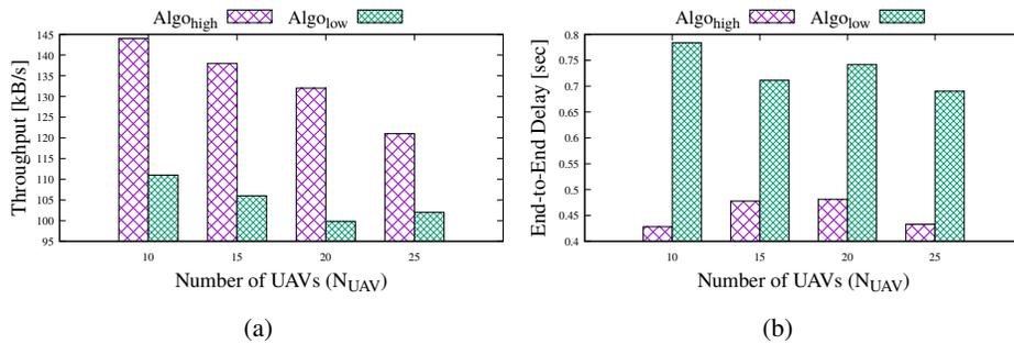
**Fig. 5.** The throughput (Figure 4(a)) and the end-to-end delay (Figure 4(b)) indexes comparing *Algo<sub>high</sub>* and *Algo<sub>low</sub>* varying the number of UAVs.
