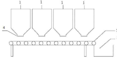
1---Weighing and blanking mechanism; 2--- Burden delivery mechanism;
