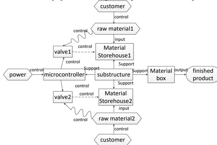
**Fig. 10.** The function model (two Material Storehouses)
