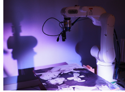
Figure 5. Experimental setup: camera mounted on a Viper 850 from ADEPT
