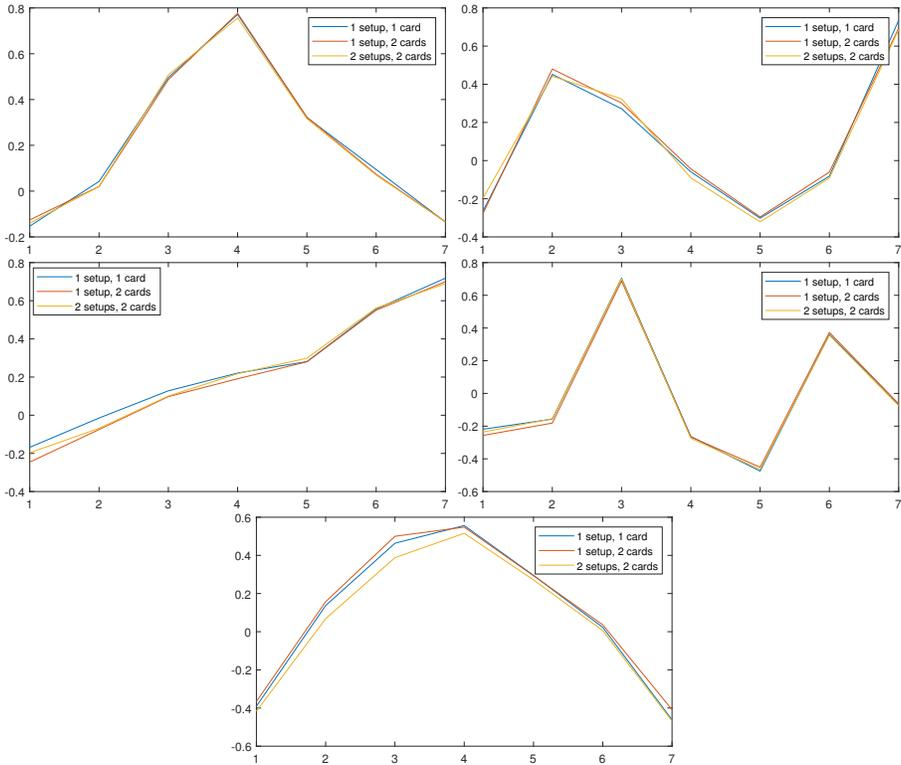
Figure 7: Mode shapes obtained with the three tests.
