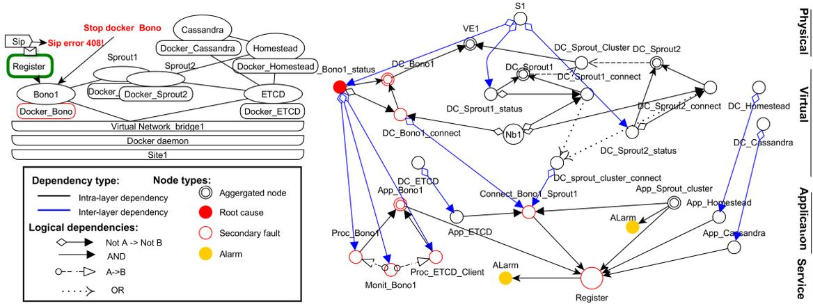
Figure 2. SAKURA RCA Fault propagation use case.
