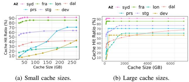
Fig. 3. Cache hit ratios of different AZs vs. shared cache size.
