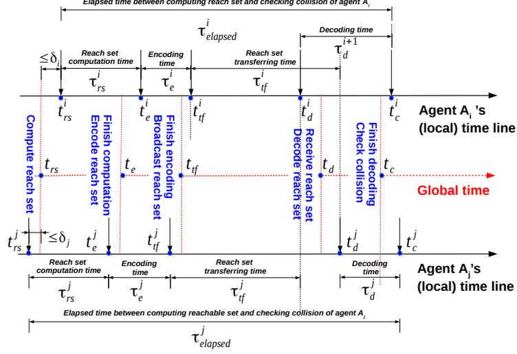
Fig. 1: Timeline for reachable set computing, encoding, transferring, decoding and collision checking.
