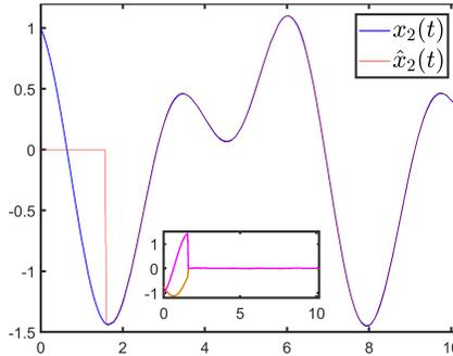
Fig. 2. Simulations of (73) with  $a_0(t) = 1$  and  $C(t) = [\max\{\cos(4t), 0\} \ 0]$ . Main Figure:  $x_2$  and its estimate  $\hat{x}_2$  with  $R_2 = 0.0204$ . Inset:  $\tilde{x}_1 = \hat{x}_1 - x_1$  (Orange) and  $\tilde{x}_2 = \hat{x}_2 - x_2$  (Pink) with  $R_2 = 0$ . Time unit on horizontal axes is seconds.
