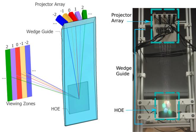
**Fig. 2.** (left) Overview of the prototype: 5 projectors labeled  $-2..2$  are coupled into a wedge light guide, and a HOE scatters the light towards independent viewing zones  $-2..2$ . (right) Photograph of our prototype from viewing zone 0
