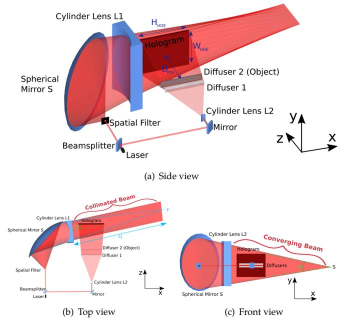
**Fig. 3.** Recording setup of the HOE. The object beam is created by a rectangular diffuser representing the viewing zone. The reference beam is created by creating a convergent beam with a spherical mirror and collimate it in one direction with a cylinder lens.
