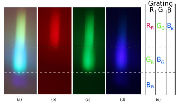
**Fig. 7.** Images of the viewing zones on a  $D_{obs}$  distant screen, created by (a) Red, green and blue wavelengths; (b) Red only; (c) Green only; (d) Blue only; (e) Illustration of the wavelength-dependent contributions of each grating.
