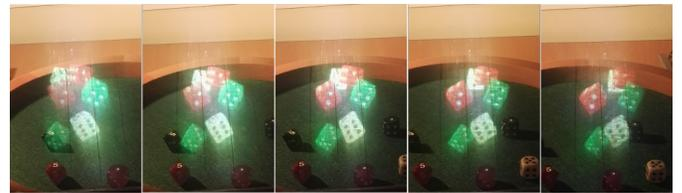
**Fig. 8.** Photographs of the display from each viewing zone. Parallax and transparency can be observed.
