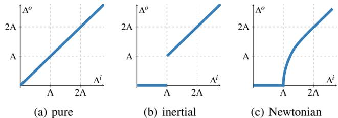
Fig. 1: Output ( $\Delta^o$ ) over input ( $\Delta^i$ ) pulse width for different delay models.
