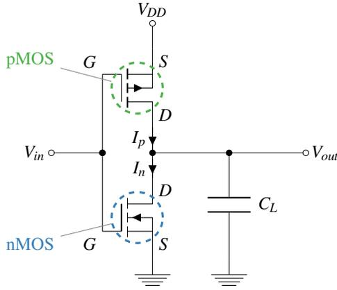
Fig. 6: Transistor level implementation of a CMOS inverter.
