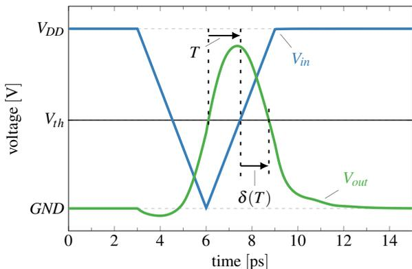
Fig. 4: Characterization procedure of *DDM*, showing the input slopes ( $V_{in}$ ) and output trajectory ( $V_{out}$ ) of an inverter gathered from *SPICE* simulations in 15 nm FinFET technology ( $V_{DD} = 0.8 V$ ).
