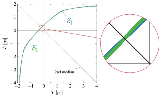
Fig. 5: Involution delay function of an inverter in 15 nm FinFET technology. Note that  $\delta_{\uparrow}$  and  $\delta_{\downarrow}$  have to meet at the second median to fulfill the involution property.
