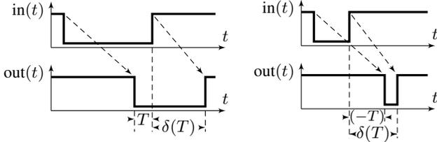
Fig. 2. Left: Input/output signal of a single-history channel, involving the previous-output-to-input delay  $T$  and the resulting input-to-output delay  $\delta(T)$ . Right: Input transition with  $T < 0$ .
