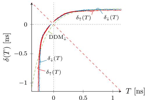
Fig. 7. Measured  $\delta_{\downarrow}$  (blue) and  $\delta_{\uparrow}$  (red) for UMC-90 inverter chain for  $V_{DD} = 0.6$  V, which support the involution hypothesis. By contrast, there is no perfect fit for the exponential DDM delay function (dashed green). From [13].
