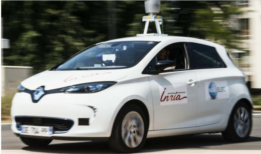
**Fig. 4.6:** Autonomous vehicle platform, Renault Zoe car, equipped with a Velodyne HDL-64 LiDAR
