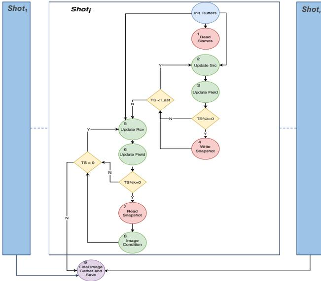
Fig. 1: Color-coded RTM flowchart for  $n$  shots: green circles represents GPU computation kernels, red (and blue) circles for I/O and memory kernels, purple circles for reduction kernels, and yellow diamonds for conditionals to trigger I/O operations.
