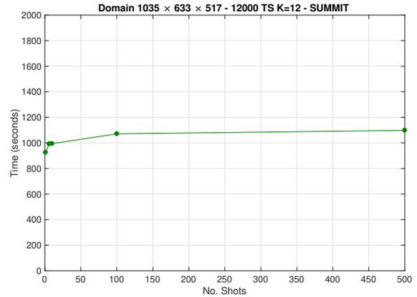
Fig. 12: Weak Scaling of a synthetic 3D model with  $K=12$  using TB-RTM OOC on Summit (1 Shot/GPU - 6 GPUs/Node).
