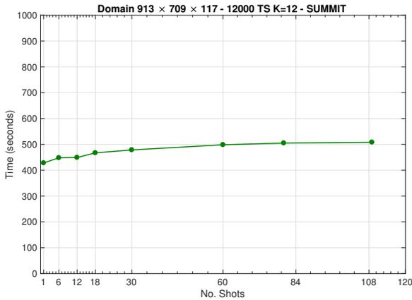
Fig. 11: Weak Scaling of Salt 3D model with  $K=12$  using TB-RTM OOC on Summit (1 Shot/GPU - 6 GPUs/Node).
