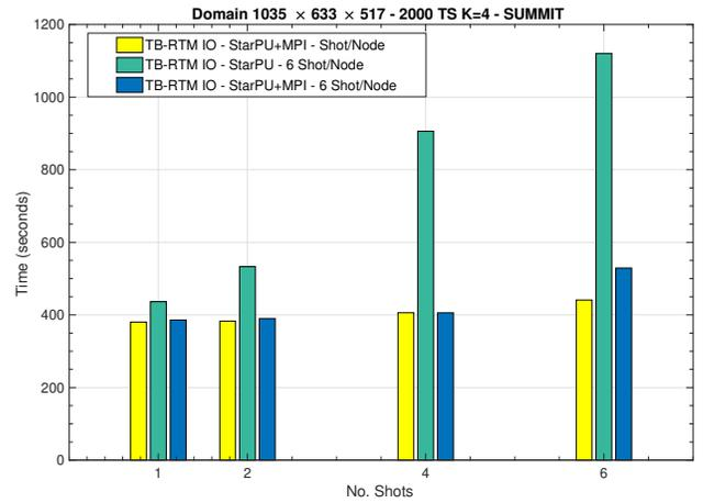
Fig. 7: Plotting STARPU +MPI and STARPU implementations of TB-RTM for simulating multiple shots RTM for  $K=4$ .
