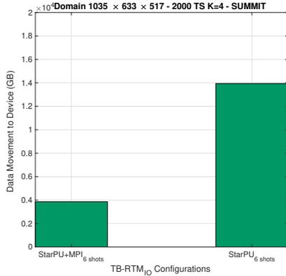
Fig. 8: Data movement from memory to device of TB-RTM IO for simulating multiple shots RTM for  $K=4$  on one node.
