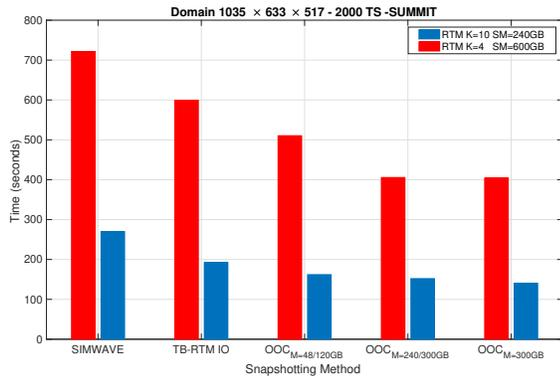
Fig. 5: Time to the solution of single shot RTM of larger size on one node of Summit (V100 GPU with NVMe) against different snapshotting methods supported in TB-RTM in addition to SIMWAVE as our baseline.
