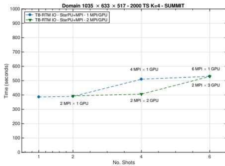
Fig. 9: Impact of pinning on time to solution TB-RTM IO for simulating multiple shots RTM for  $K=4$  on one node.
