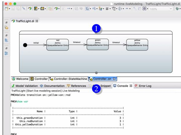
Fig. 4: User interface of Live-UMLRT
