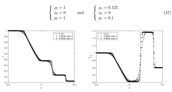
Figure 1: Comparison between exact and P-BGK solutions for  $\gamma = 5/3$ . Density (left) and Temperature (right) profiles. First and second order scheme.
