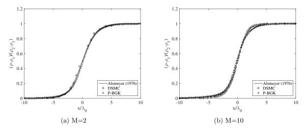
Figure 6: Density profiles obtained with DSMC, experiments and the P-BGK model.
