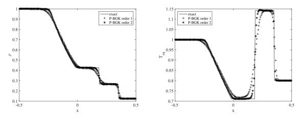
Figure 2: Comparison between exact and P-BGK solutions for  $\gamma = 7/5$ . Density (left) and Temperature (right) profiles. First and second order scheme.
