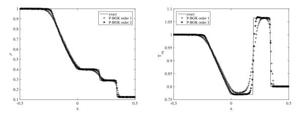
Figure 4: Comparison between exact and P-BGK solutions for  $\gamma = 9/7$ . Density (left) and Temperature (right) profiles. First and second order scheme.
