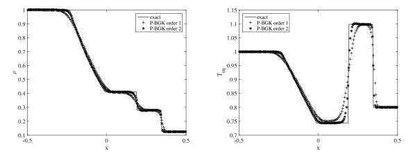
Figure 3: Comparison between exact and P-BGK solutions for  $\gamma = 4/3$ . Density (left) and Temperature (right) profiles. First and second order scheme.
