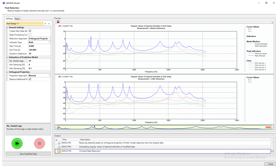
Figure 5: Removal harmonic at 370 Hz. Burst sine: 370Hz, 10s.
