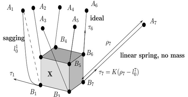
Fig. 1. A CDPR and various cable model
