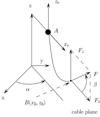
Fig. 2. Notation for a sagging cable
