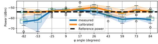
Fig. 4. Boxplot of the calibration results. Each of the 10 shown values of  $\varphi$  is tested with 10 random values of  $\theta$ . A total of 100 orientations were evaluated. The calibrated signal (in orange) is less variable, and close to the reference power than the raw signal (in blue).
