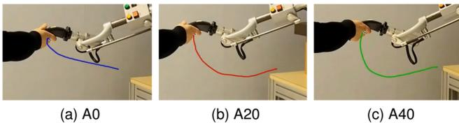
Fig. 4. User trajectory for a reaching movement for the three weightings A0 (blue), A20 (red), and A40 (green). In A0, only  $\mathcal{H}_r$  is considered, and the user trajectory is therefore almost horizontal. As the contribution of  $\mathcal{H}_{\mathcal{W}}$  to the haptic feedback increases, the trajectory tries to minimize the user discomfort by moving the arm to a downward (more comfortable) position.
