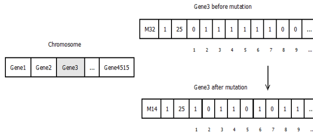
Fig. 3: Example of a mutation operation
