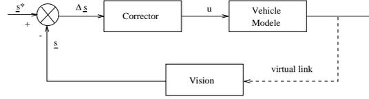
Fig. 2. Visual servoing scheme in  $H_\infty$  space
