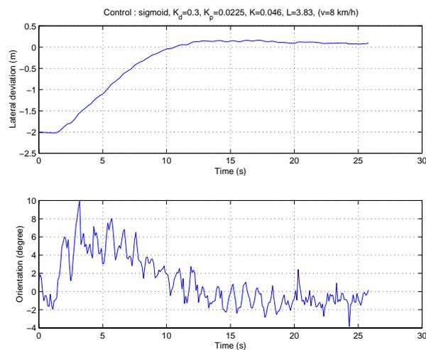
Figure 6. experimental results on the combine harvester
