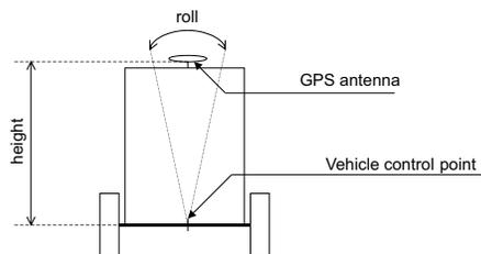
Figure 7. roll effect on the antenna position
