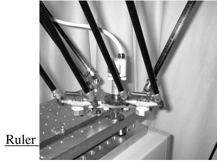
Fig. 5 : Validation experiment - Kinematic constraint on the end-effector
