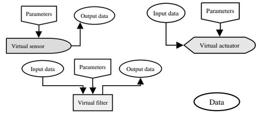
Fig. 3. Basic components of the FBA architecture.
