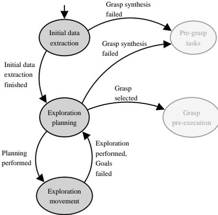
Fig. 4. Automata-based description of the grasp-synthesis task.
