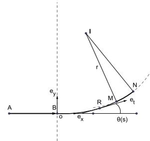
Fig. 4. Connection with an arc of clothoid
