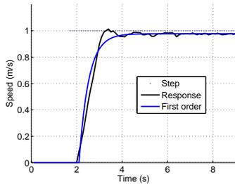
Fig. 11. Longitudinal step response: identification with 1<sup>st</sup> order
