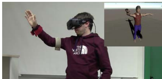
Fig. 1. The orientation of the user’s arm is tracked wearing two armbands, one at the forearm and one at the upper arm.
