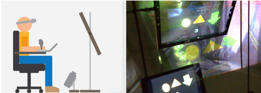
Fig. 5. To the left, a schematic picture of the CAVE simulation room and its primary components. To the right, a photo that shows all three display solutions at once (the simulation only showed one at a time)
