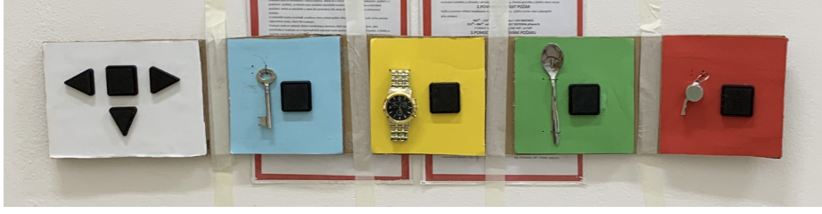
Fig. 3: Design C – lo-fi prototype introducing a tactile cursor providing information about the surrounding and current location. The panel with key symbol served to navigate the user back to the room. Other three panel's function did not change.
