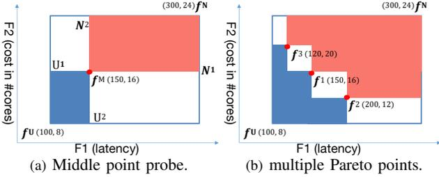
Fig. 2. Uncertain space in 2D (latency, cost) space for TPCx-BB Q2.  $f^U$  and  $f^N$  are the Utopia and Nadir points, respectively. In (a),  $f^M$  is the solution to the middle point probe. In (b),  $(f^1, f^2, f^3)$  represent the solutions of a series of middle point probes.
