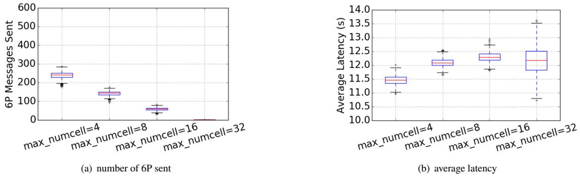
**FIGURE 5** *Bursty traffic, using Advanced MSF.* Number of 6P messages sent by Mote 4 (*left*) and end-to-end latency (*right*). Plots only for Mote 4. Comparing to regular MSF (Fig. 4), end-to-end latency is equivalent, but the number of 6P messages is halved.
