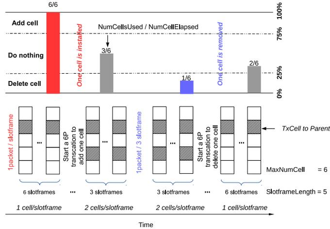
**FIGURE 1** MSF adapts the number of cells a mote allocates to a neighbor according to the number of frames they exchange. Here,  $\text{MAX\_NUMCELL} = 6$ . A cell is added when the cell usage is over 75%, and deleted when below 25%.
