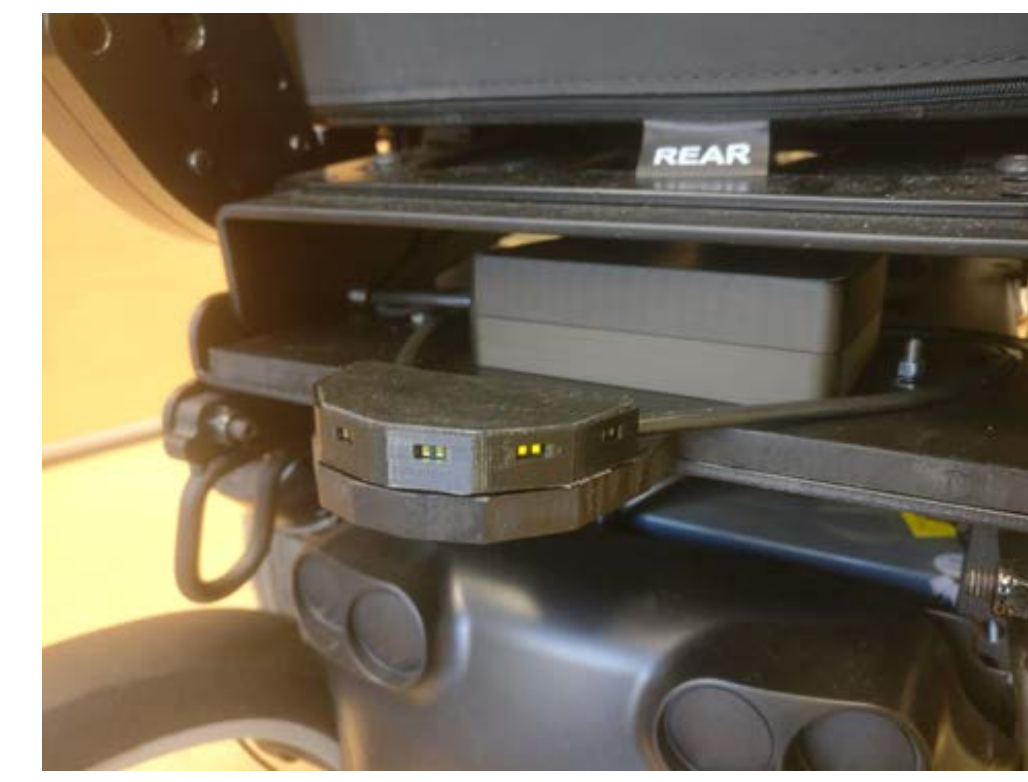
a prototype anti-collision system based on Infra Red technology and algorithms for a low cost solution
