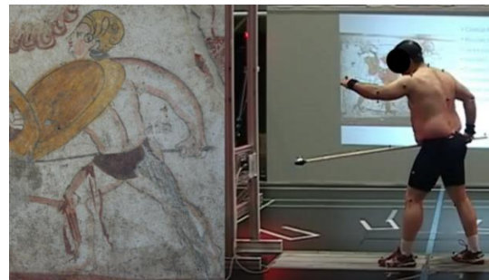
Figure 1 – (left) Sample icon representative of a plausible low posture, low targeted zone and spear attack. (right) Initial posture of one trial, developed from the icon. The subject is hitting a force sensor, and is equipped with motion capture markers.
