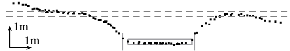
Figure 11. Risk of false detection due to horizontal road sides at the same height: the dashed height interval may contain more points than the plateau but it is split in two disconnected sets.
