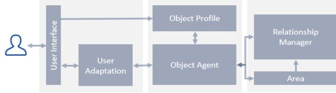
**Fig. 1.** Main Components of the DANOS Framework
