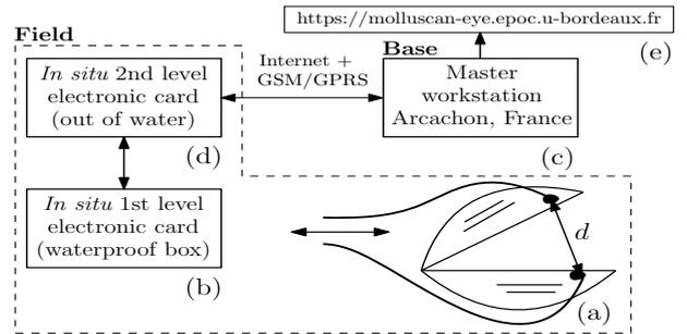
Fig. 1. Schematic representation of the HFNI valvometer
