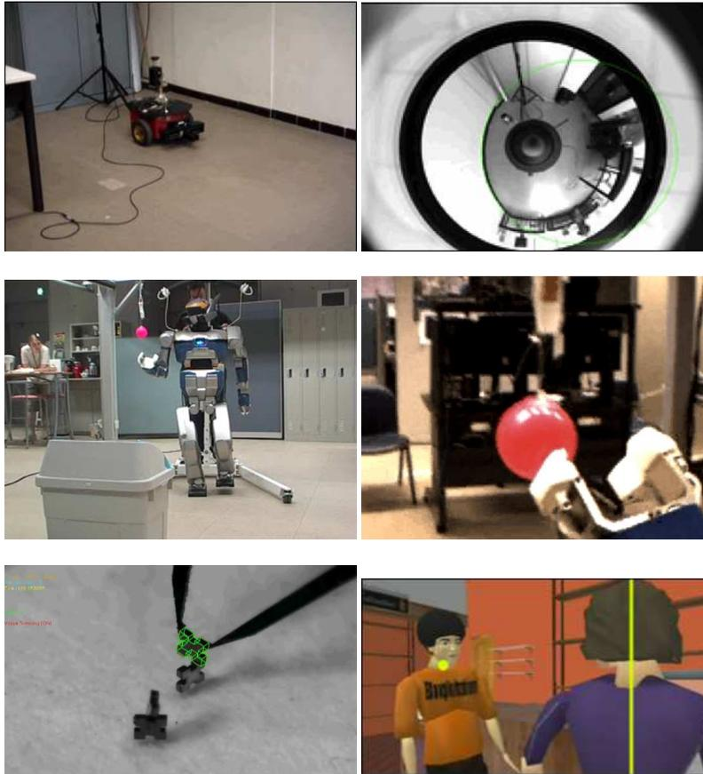
**Fig. 4** Few applications of visual servoing: navigation of a mobile robot to follow a wall using an omnidirectional vision sensor (top line), grasping a ball with a humanoid robot (middle line), assembly of MEMS and film of a dialogue within the constraints of a script in animation (bottom line).
