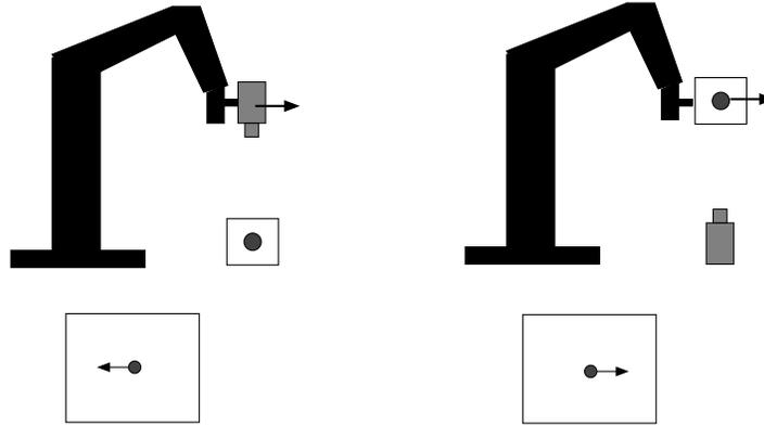
**Fig. 3** In visual servoing, the vision sensor can be either mounted near the robot end-effector (eye-in-hand configuration) or outside and observing the end-effector (eye-to-hand configuration). For the same robot motion, the motion produced in the image will be opposite from one configuration to the other.
