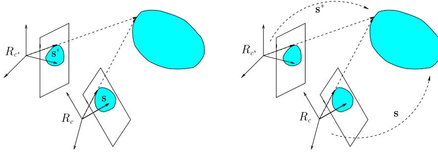
**Fig. 2** If the goal is to move the camera from frame  $R_c$  to the desired frame  $R_{c^*}$ , two main approaches are possible: IBVS on the left, where the features  $\mathbf{s}$  and  $\mathbf{s}^*$  are expressed in the image, and PBVS on the right, where the features  $\mathbf{s}$  and  $\mathbf{s}^*$  are related to the pose between the camera and the observed object.
