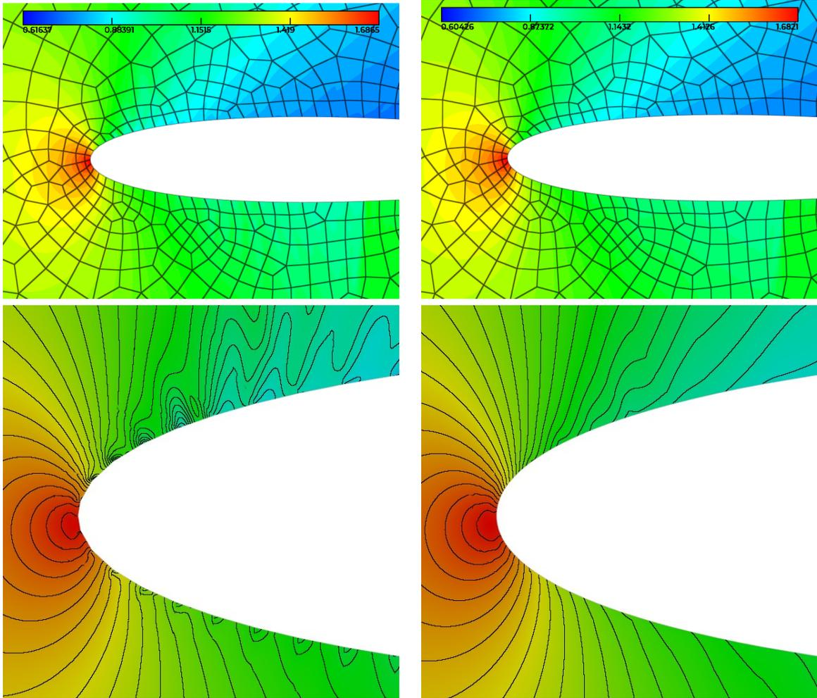
Figure 3: Degree 5 resolution of the Euler equations on a NACA0012 airfoil with a  $Q^1$ -mesh (left) and with a  $Q^2$ -mesh (right). Mesh edges are shown in black and filled iso values (top) and with darkened isolines (bottom) are displayed and show the inaccuracy in the linear representation of the geometry near the leading edge. Courtesy of Christophe Peyret (ONERA).
