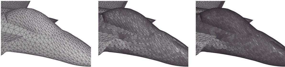
Figure 27: Left, zoom on a curved part of the  $P^3$ -mesh used for the BEM resolution. Middle and right, various tessellation levels used for the display of the geometry. Courtesy of Stéphanie Chaillat (ENSTA).
