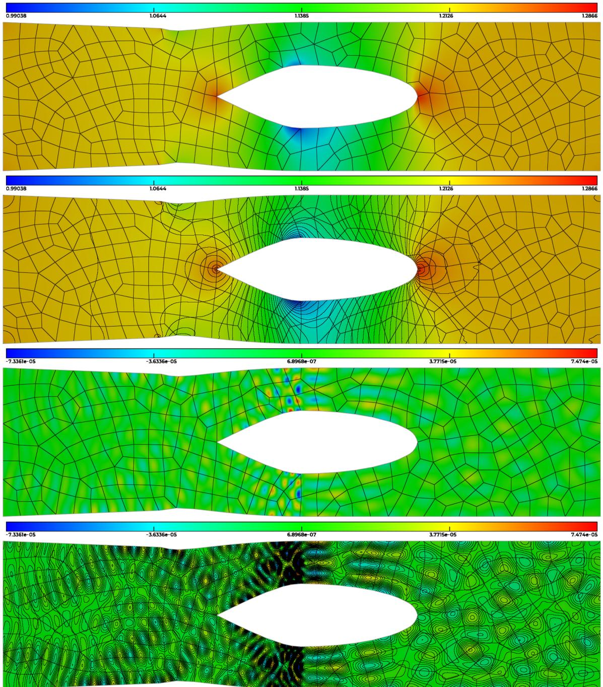
Figure 30: Top (two first pictures), mean flow around an engine using a  $Q^2$  mesh with  $Q^{10}$  solution. Bottom (two last pictures), perturbation over the mean flow using a  $Q^8$  solution. Courtesy of Christophe Peyret (ONERA).
